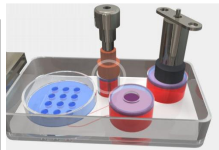
Figure 2. Valve for fluidic control and sampling compartment for pH measurements
